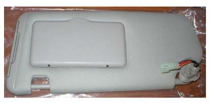
This isn't a problem, we'll just use the two-wire black harness off the OEM visor and attach it to the new Homelink visor so it will plug back in to the factory harness in the roof.
