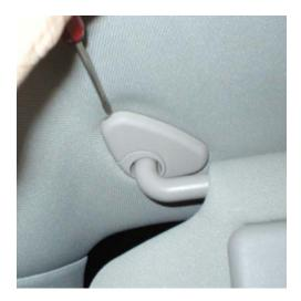
Now you will have access to the two screws holding the visor in place.
