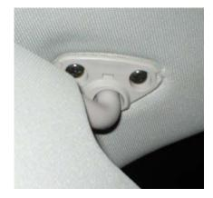
Using the #2 Phillips Screwdriver remove both the screws with one hand while holding the visor in place with the other. Once both the screws are out, gently pull the visor away from the roof. You will see the harness for the lighted vanity mirror, unplug it so you can remove the entire sun visor.
