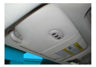
With the ignition "On'" or set to "Acc" you can test the vanity Mirror by opening it, lights should come on. Test the HomeLink by pressing any of the buttons, the red indicator should light up.
