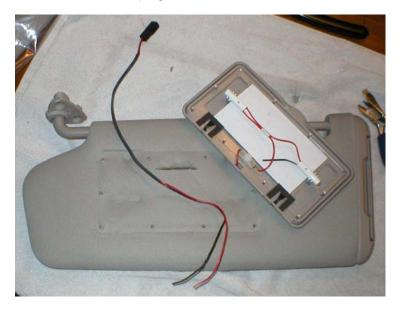
Cut the wire to about 4" off the harness, then strip the red and the black wire back about 1/8".
