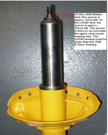
The parts you **WILL** be able to use off the USDM front struts are: the dust boot, the upper spring cushion, the upper perch and the nut to hold it all together. You **WILL NOT** be able to use the USDM bump stop...but that's OK, inverted struts (like these Bilstein's) don't use one.
