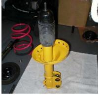
Then put the spring in place (you will need to use a spring compressor at this point), place the USDM upper spring perch in place (position it properly) with the rubber isolator in place, place the Spec B strut mount in place and secure it all together with the 17mm nut and your all set! Position it in the car and secure all the bolts to the specified torque.
